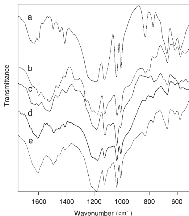
Figure 6 FTIR spectra of (a) SPS (b) POA/SPS (c) POP/SPS (d) PMA/SPS, and (e) PMP/SPS complexes.
